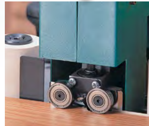
Power trimming unit: trimming both sides simultaneously.
