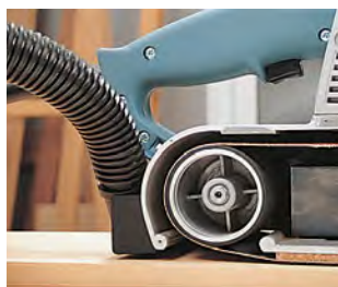
External dust collector connection on model LB31E.
