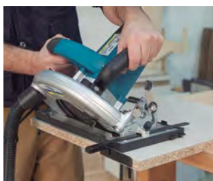
Performs cuts of up to 75 mm.
