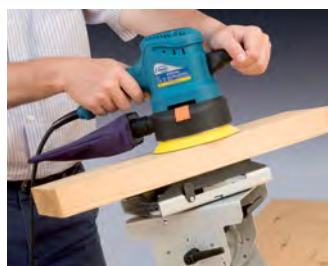
Folding and rotary adjustable support.
