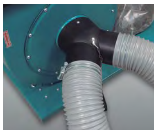
With two sockets, it includes 2 tubes of Ø 100 mm.
