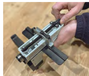
Micrometric regulation of the cutting width.
