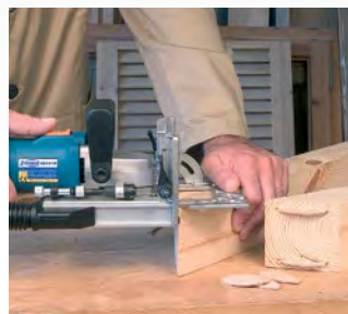
Stronger joints with No. 6 splines.
