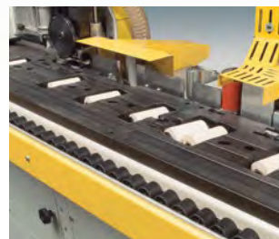
Equipped with auxiliary rollers on the banding table and a presser assembly, to achieve the optimum pressure of the panel against the banding unit. This ensures a correct banding.
