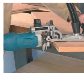
Trimming the edge with the straight bit.
