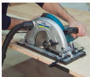
Performs cuts of up to 75 mm.
