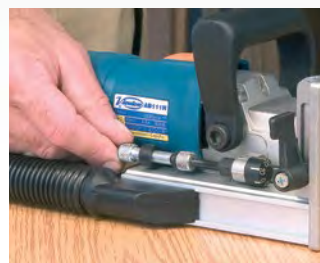
Quick adjustment of different slotting depths.
