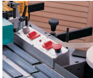
Safety control (STOP). Electronic temperature control.
