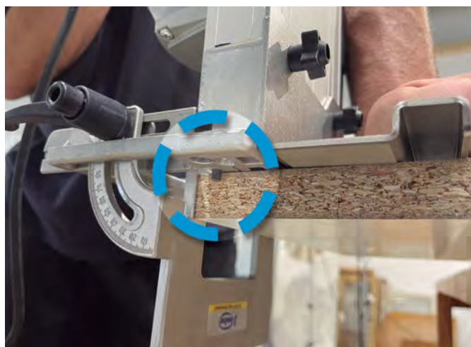
Automatic positioning system of retractable stoppers.
