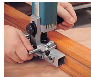
Slotting a window, lock side.
