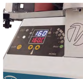
Temperature adjustment (120 to 200°C) controlled by microprocessor for higher accuracy on measurement. Temperature is rising by impulses, which protects the heating elements and increasing their working life.
