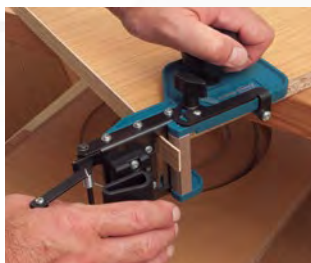
Cutting on both sides on straight panels.
