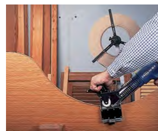
Enables banding of circular or shaped pieces.
