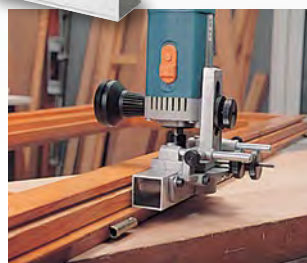
Slotting a window, hinges side.
