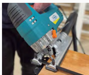
Base can be tilted from 0° to 45°.
