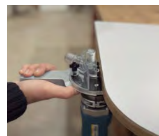
The SA100 can also be transformed into a handle for the FR156N.
