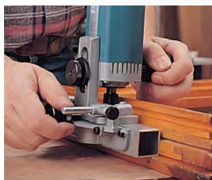
Slotting a window, flashing side.
