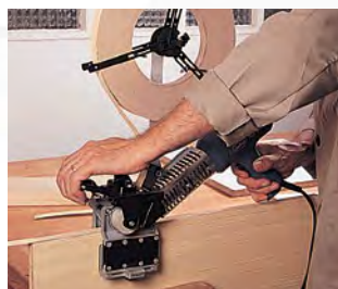
High precision and stability during edgebanding.
