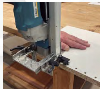
Multi-drilling Ref. 7946704 (included) With multi-drilling positioning stopper (pitch 32).
