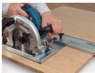
Working with 7446879 support and UCP90 guide, both optional.
