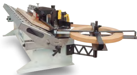
5046705 RP80 presser + support (for MEB250A).
